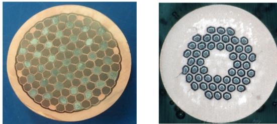
Nb<sub>3</sub>Sn conductor by JASTEC & Furukawa
