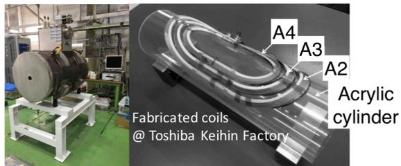
HTS 3T Dipole with COS $\theta$  windings
