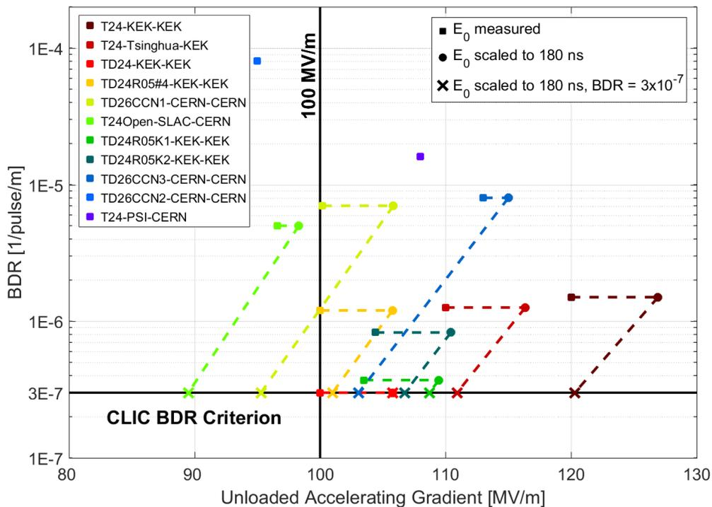
Figure 6: The performance of X-band structures can be characterized as achieved gradient (MV/m) at a given breakdown down rate (BDR/pulse/m) at the appropriate pulse-length (180ns)
