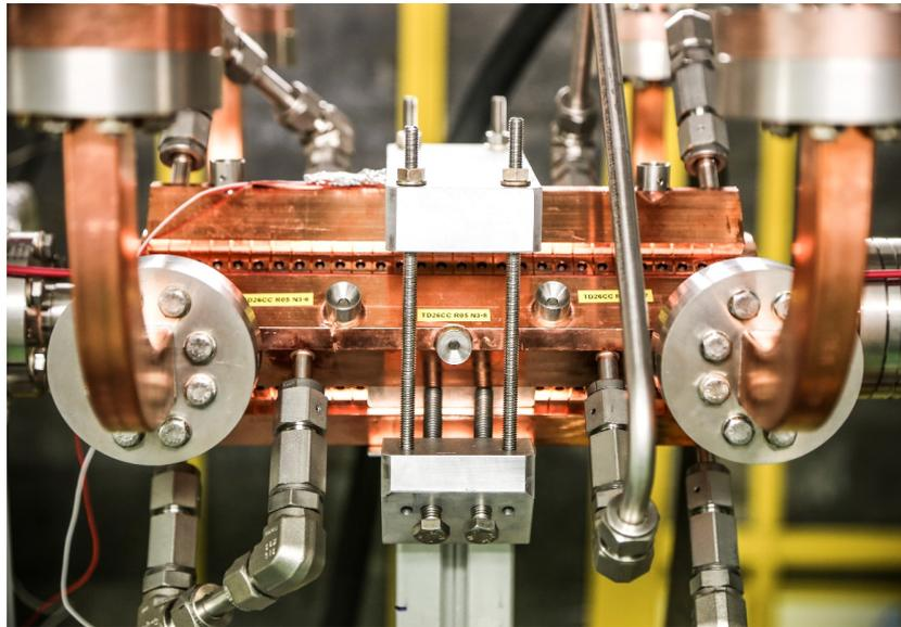
Figure 4: Xband RF structure
